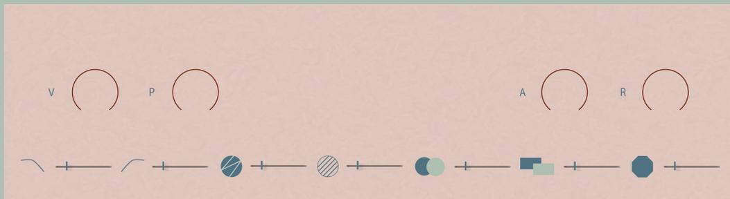
Legato Cello is a simplified version of our Stone interface. The four knobs control Volume, Pan, Attack and Release. At the bottom of the UI are the effects section to process the sound
